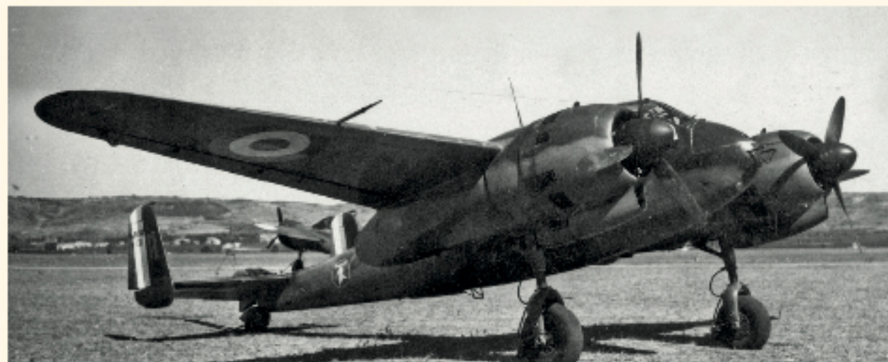
Breguet 693 n° 1011, seen here just after the armistice. It has no cannon, which indicates that its hull was completely built in Bourges, as this corresponds to the definition of the Breguet 696.
